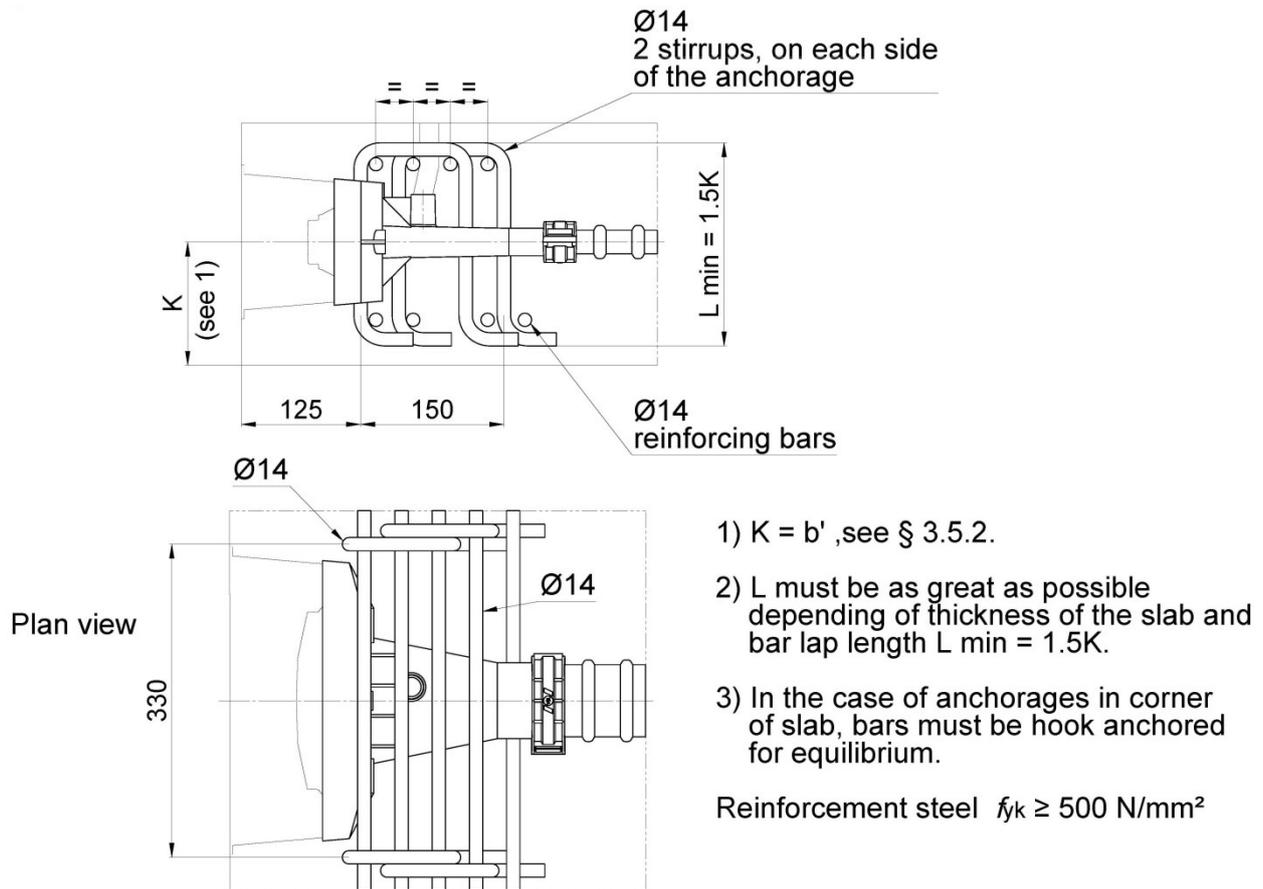
**Figure 77 Example of additional reinforcement to combine with main one type S 6-4  $f_{c,min}(t) > 16/20 \text{ N/mm}^2$**
