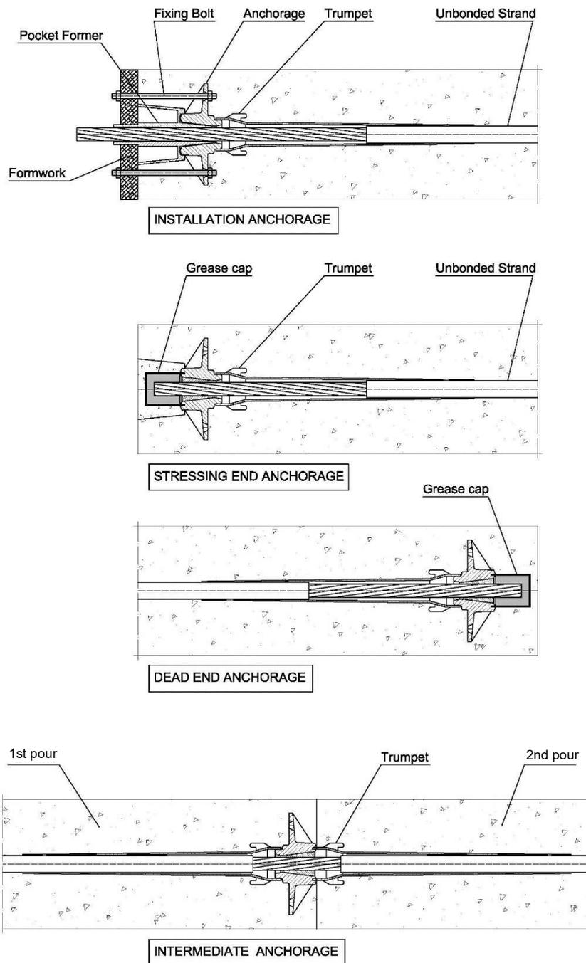
Figure 63 Anchorages type S 6-1 Standard - Unbonded system
