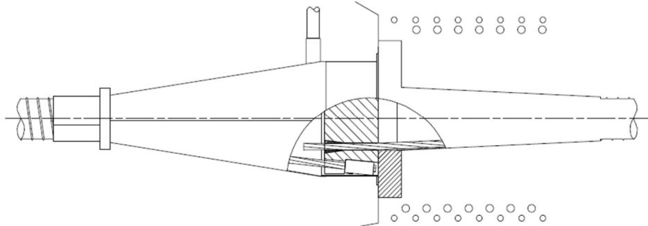
**Coupler type K with anchorage type CS**
