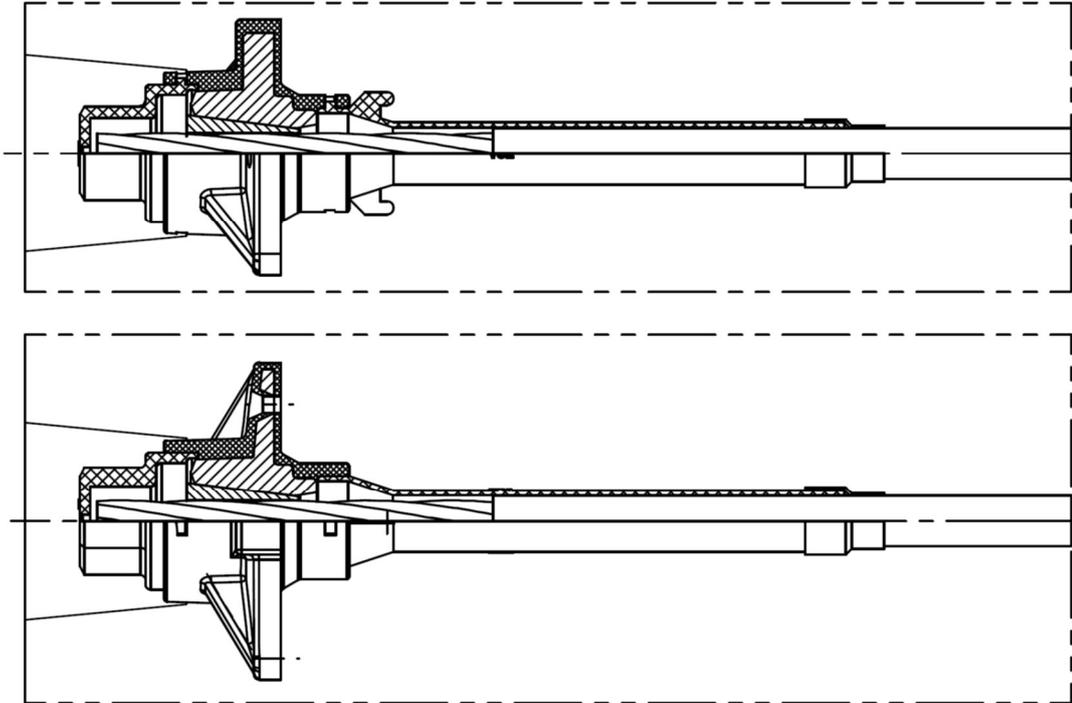
**Figure 59 Anchorage type S 6-1 PLUS - Unbonded system**
