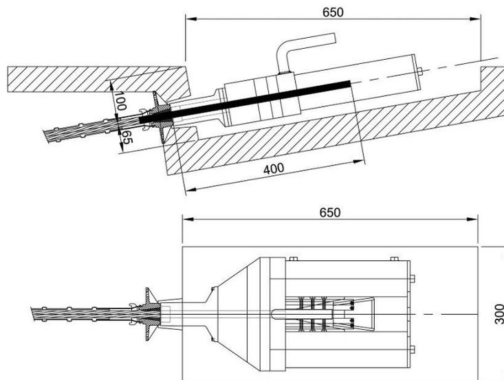
**Figure 83 Clearance requirements with Twin jack 25T**
