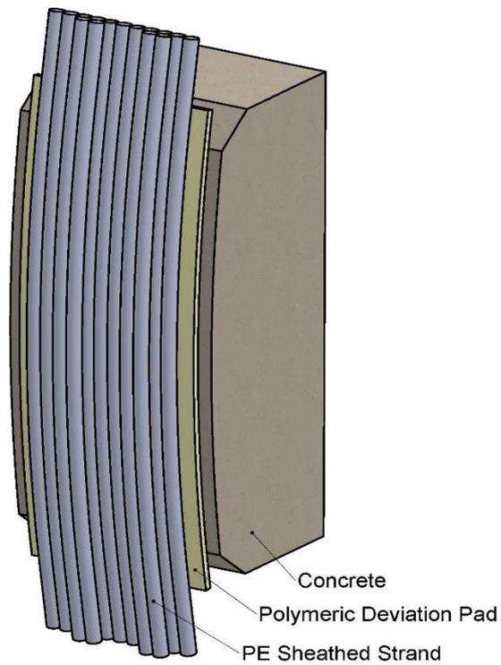
**Figure 17 Deviator E-WT- Curved deviator**
