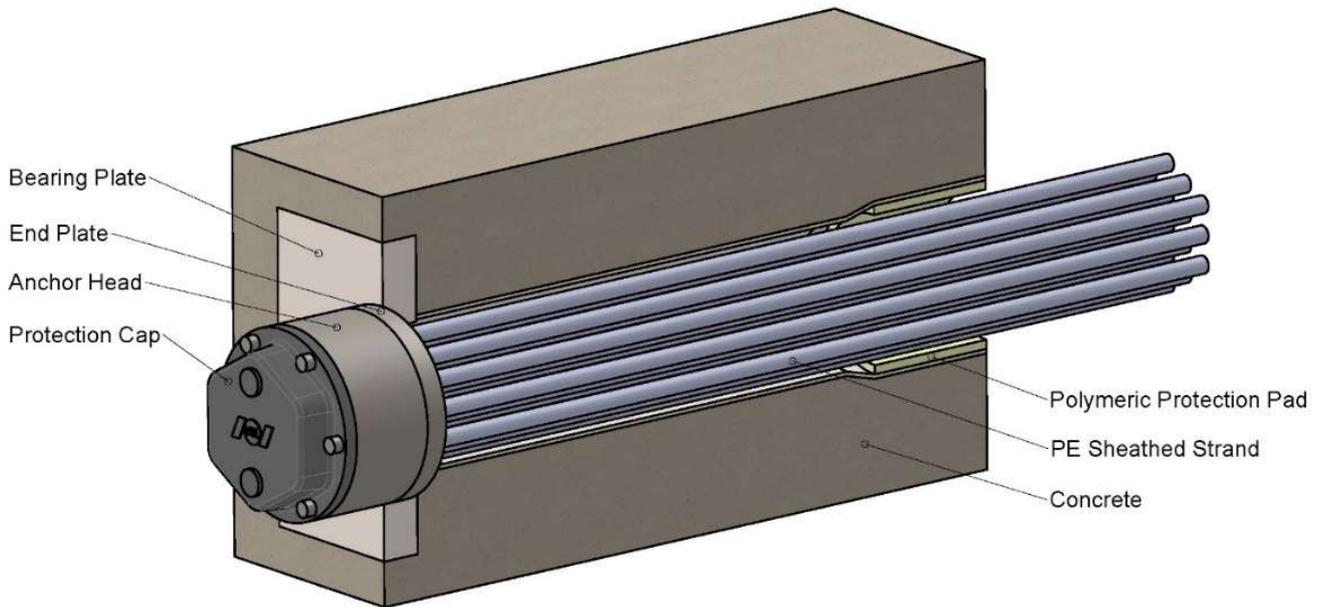
**Figure 14 Anchorages type E-WT (External unbonded tendons)-
