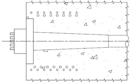
Anchorage placed against concrete structure
