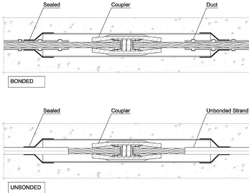
Figure 67 SK 6-1 SL Spring loaded coupler ( bonded and unbonded application )
