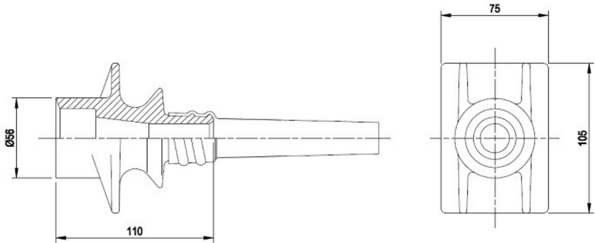
**Figure 57 Anchorages type S 6-1 - Dimensions**
