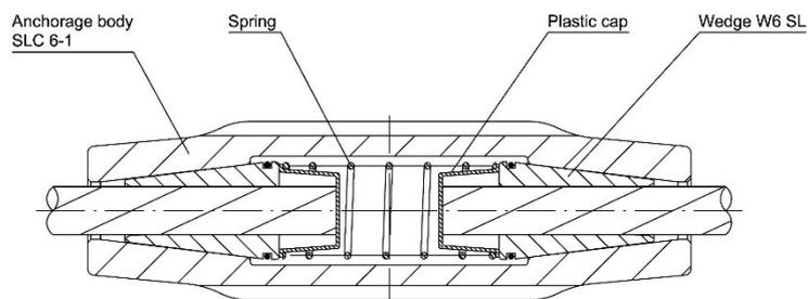
Figure 69 SK 6-1 SL Spring loaded coupler assembly drawing
