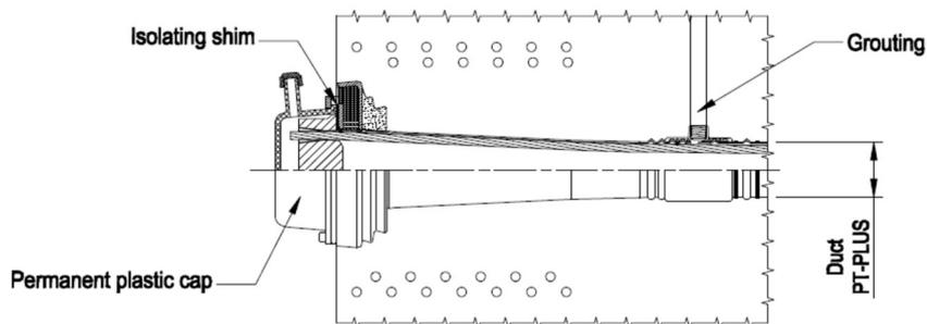
Figure 30 Arrangements anchorage type CS cast in concrete structure
