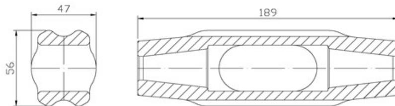
Figure 68 SK 6-1 SL Spring loaded coupler body dimensions
