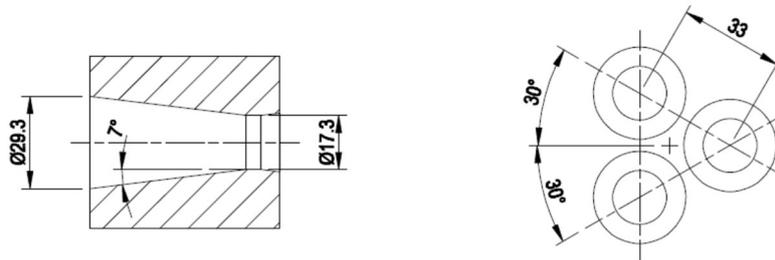
**Figure 5 Hole detail anchor head type E**
