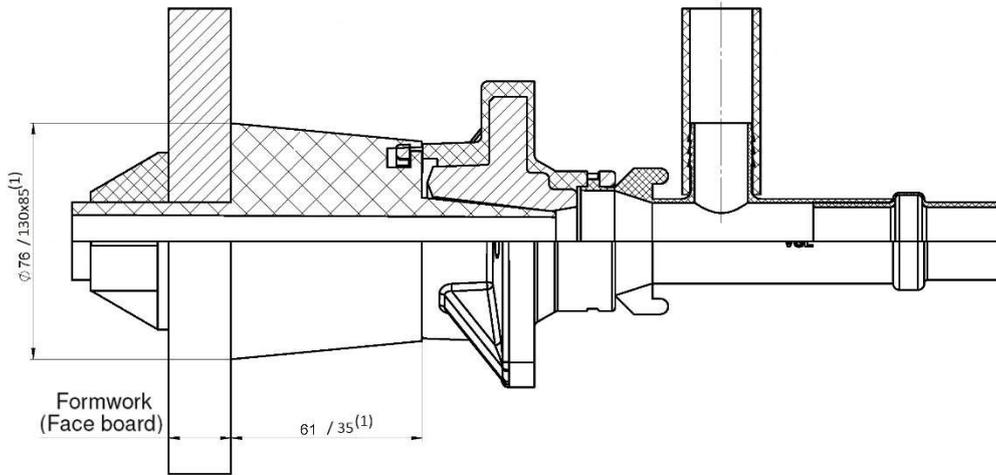
**Figure 62 Anchorages type S 6-1 PLUS – Dimensions of placing devices**
