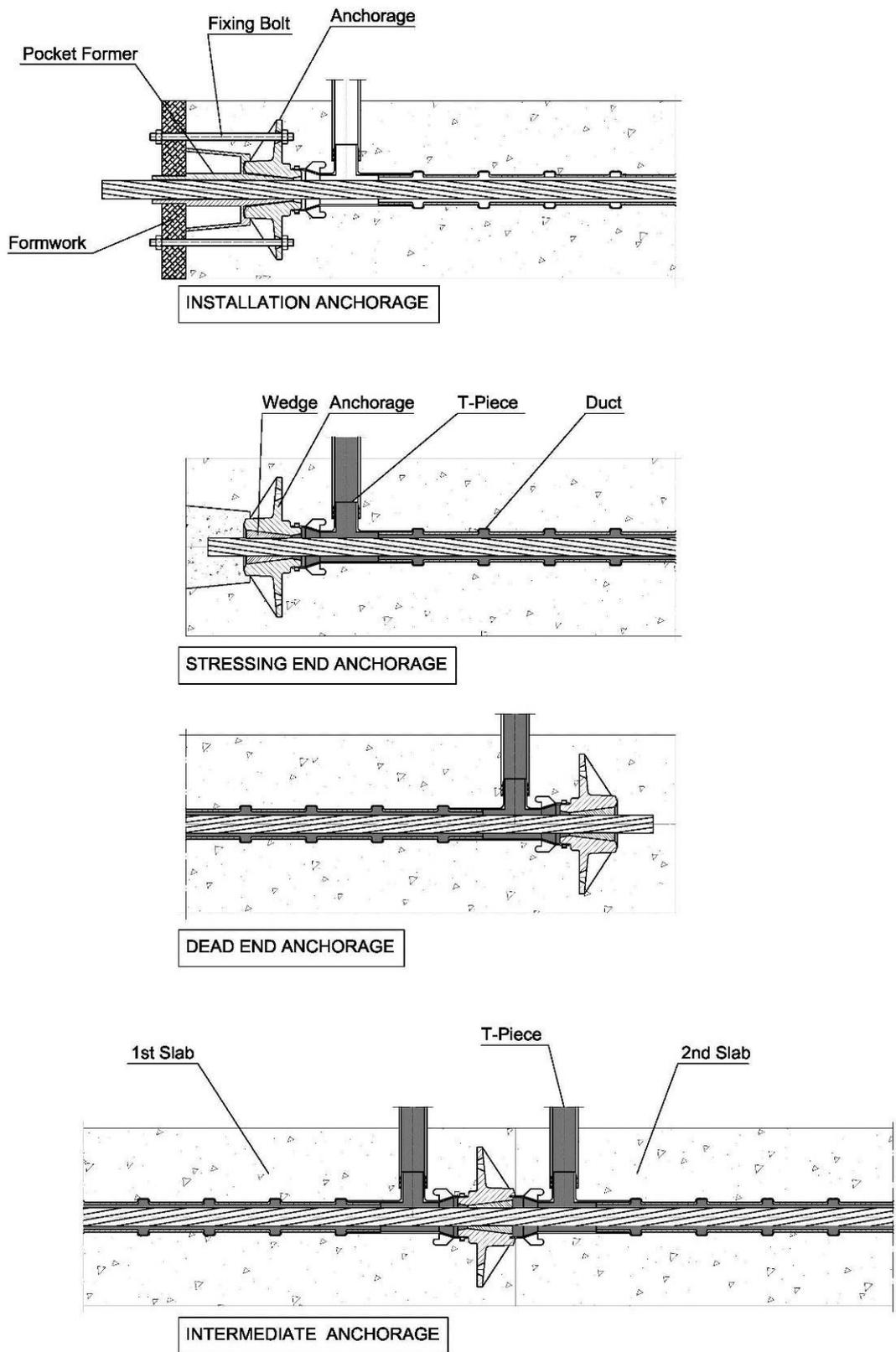
**Figure 64 Anchorage type S 6-1 Standard - Bonded system**
