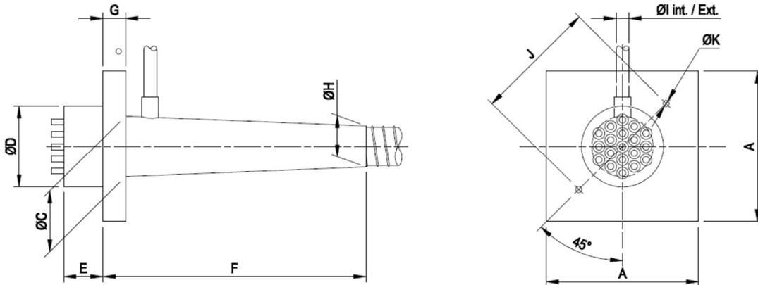
Figure 19 Anchorages type E @ 32/40 and 36/45 MPa dimensions
