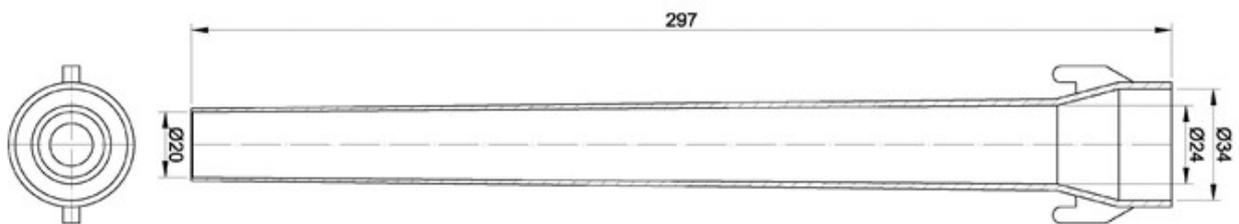
**Figure 66 Sleeve S 6-1 Standard (for unbonded application)**
