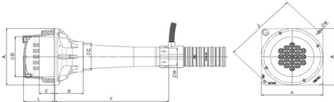
Figure 37 Anchorages type GC electrically isolated tendons dimensions
