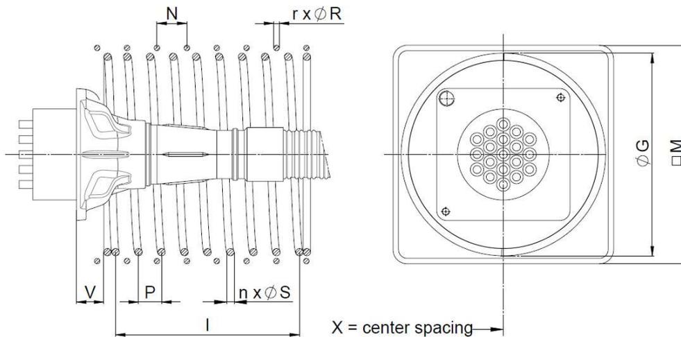
Figure 38 Local anchorage zone reinforcement type GC internal bonded post-tensioning
