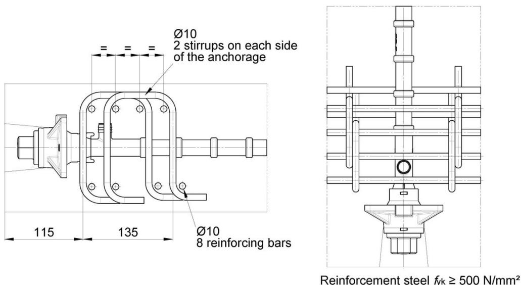
Figure 75 Example of additional reinforcement to combine with main one type S 6-1 PLUS and S 6-1 Standard  $f_{c,min}(t) > 16/20 \text{ N/mm}^2$
