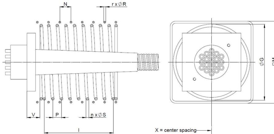
Figure 25 Local anchorage zone reinforcement type E @ 23/28 MPa
