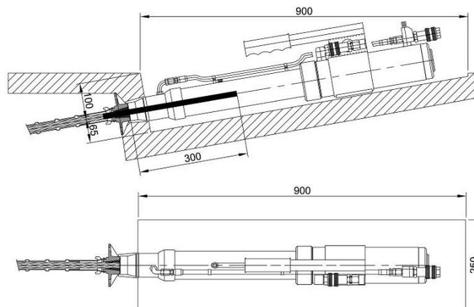
**Figure 84 Clearance requirements with jack Alevin A7-24**
