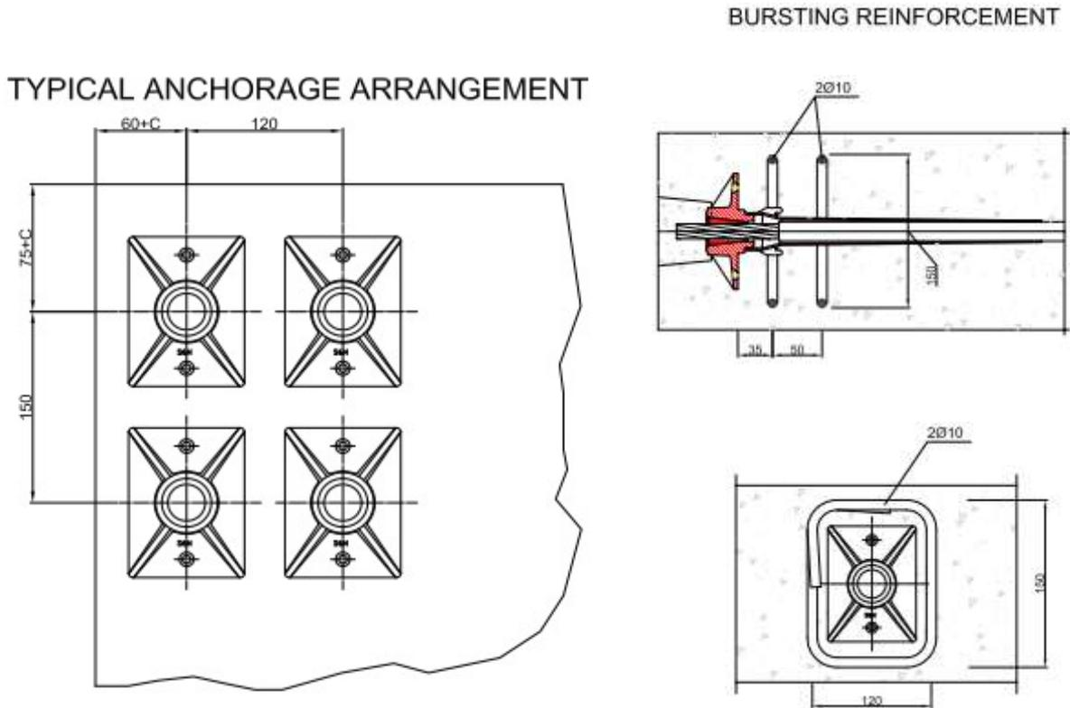
**Figure 76 Example of additional reinforcement to combine with main one type S 6-1 PLUS and S 6-1 Standard  $f_{c,min}(t) > 20/25 \text{ N/mm}^2$**
