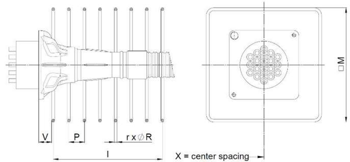
**Figure 39 Local anchorage zone reinforcement type GC external and electrically isolated tendons**
