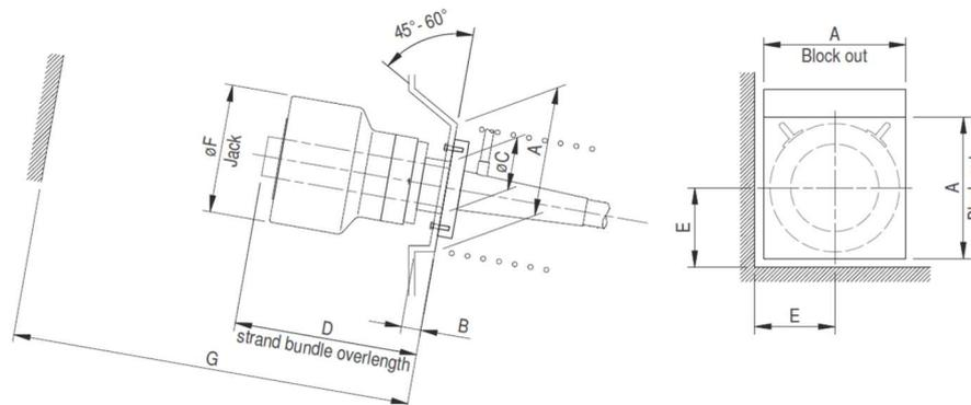
Figure 49 Block-out dimensions – Clearance requirements
