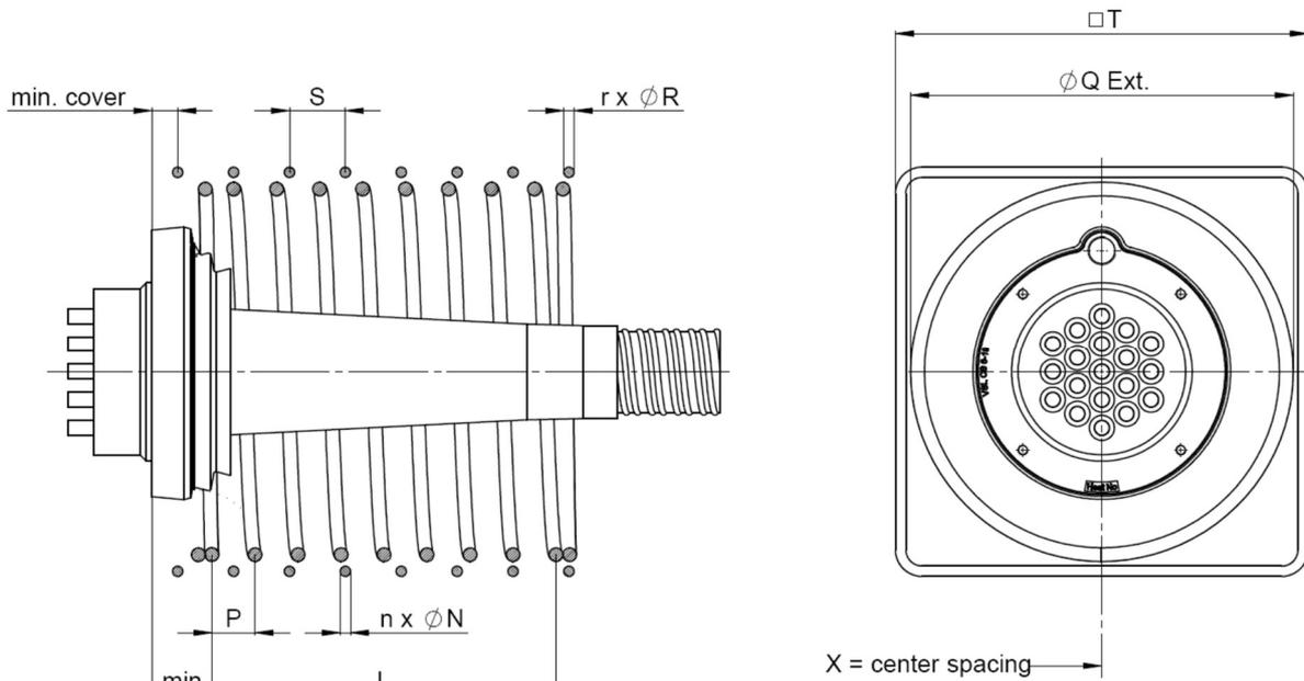
**Figure 33 Local anchorage zone reinforcement type CS @ 28/35 MPa**
