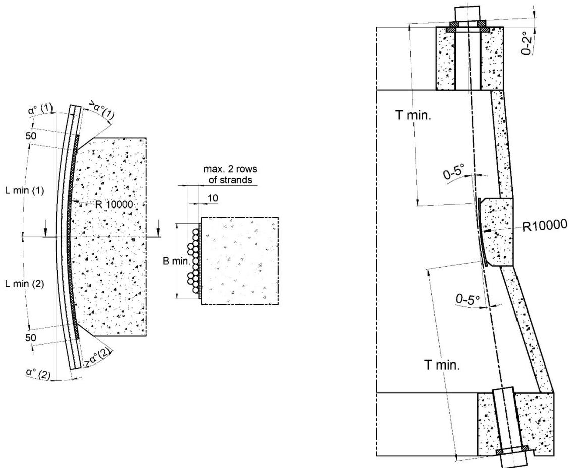
**Figure 24 Deviator E-WT – Curved deviator - Geometry and dimensions**
