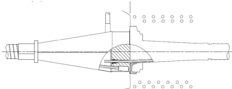
**Coupler type K with anchorage type GC**
