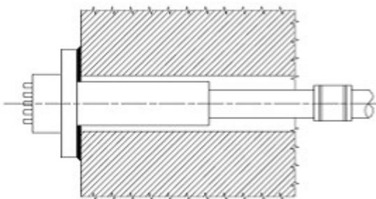
Anchorage with EP anchor head
