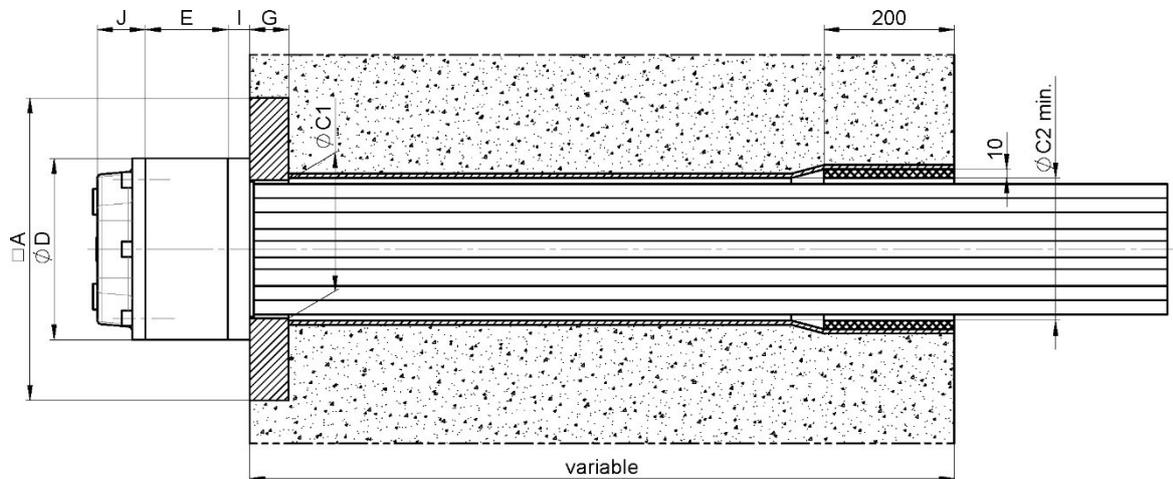
Figure 21 Anchorage type E-WT - Arrangement without shim plate - Dimensions
