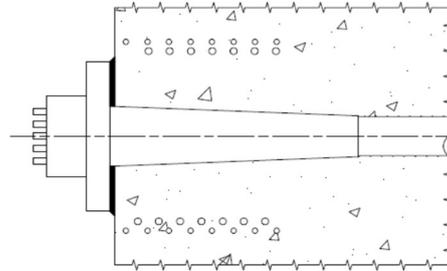
Anchorage inserted in masonry structure
