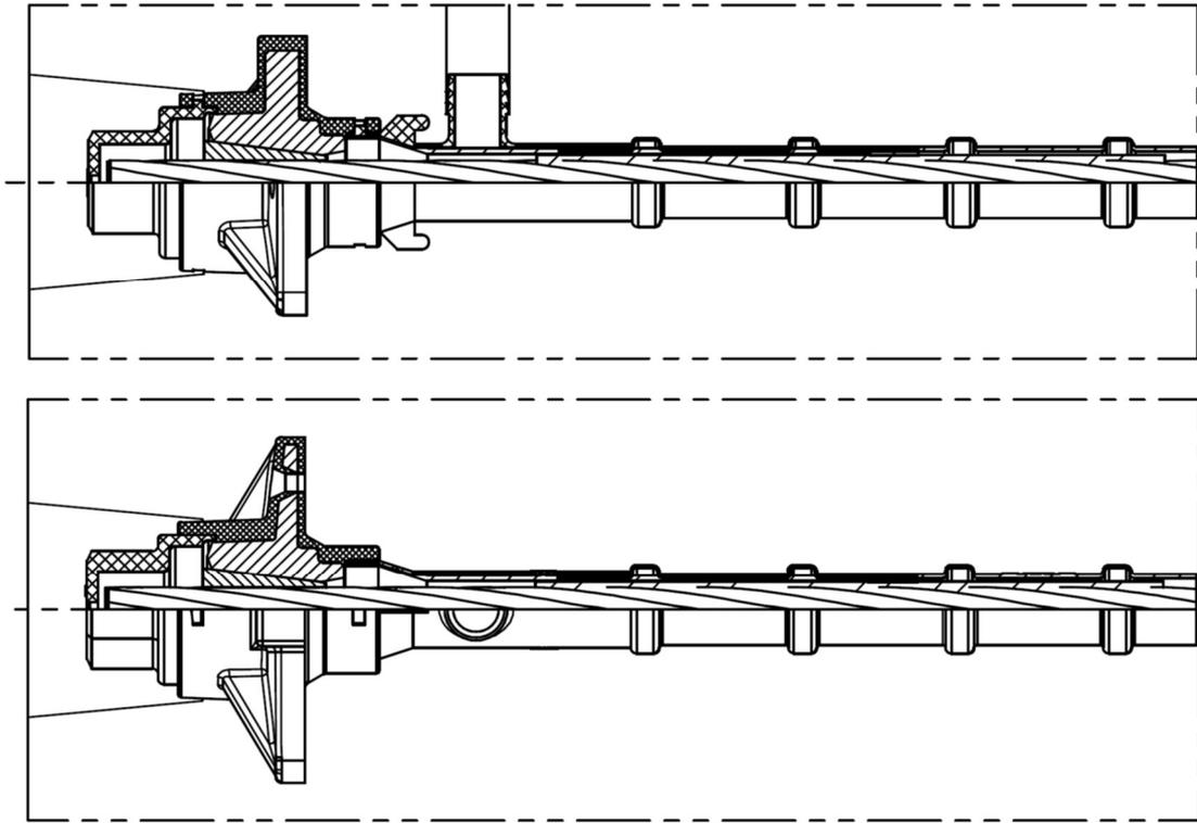
**Figure 60 Anchorage type S 6-1 PLUS - Bonded system**
