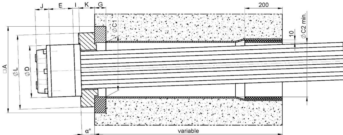
**Figure 22 Anchorage type E-WT - Arrangement with shim plate - Dimensions**
