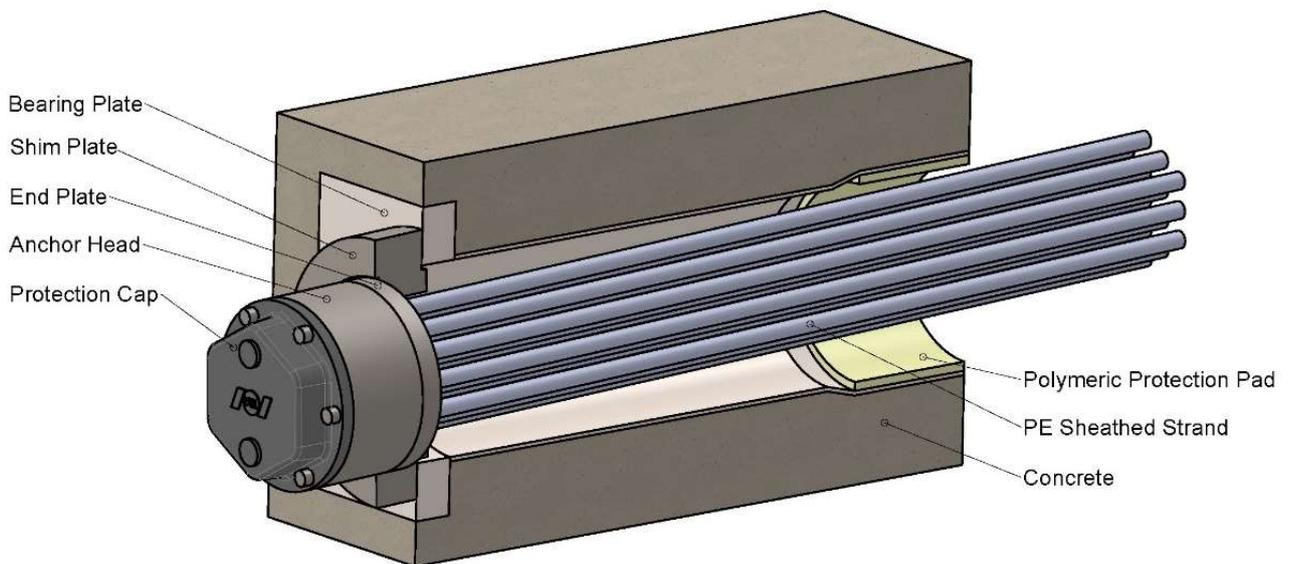
**Figure 15 Anchorages type E-WT (External unbonded tendons)-
