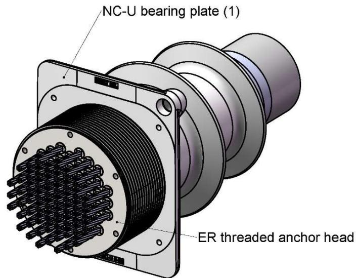
**Figure 41 Assembly with threaded anchor head for load monitoring**
