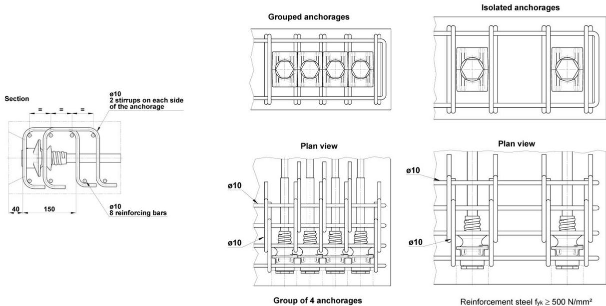
Figure 74 Example of additional reinforcement to combine with main one type S 6-1  $f_{c,min}(t) > 16/20 \text{ N/mm}^2$
