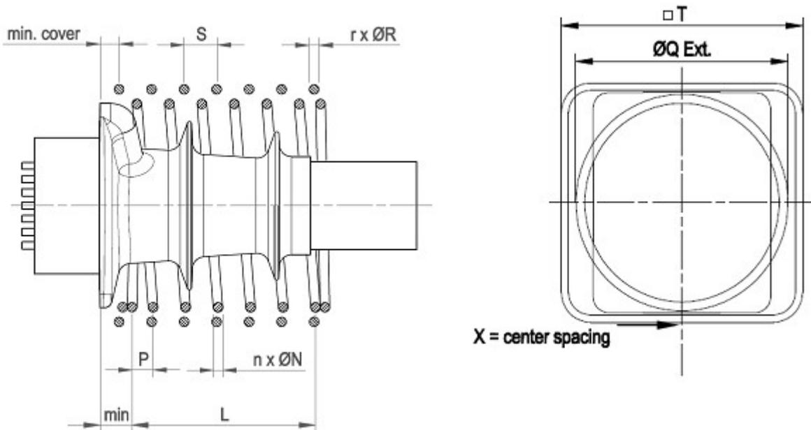
**Figure 43 Local anchorage zone reinforcement type NC and NC-U @ 53/64 MPa**
