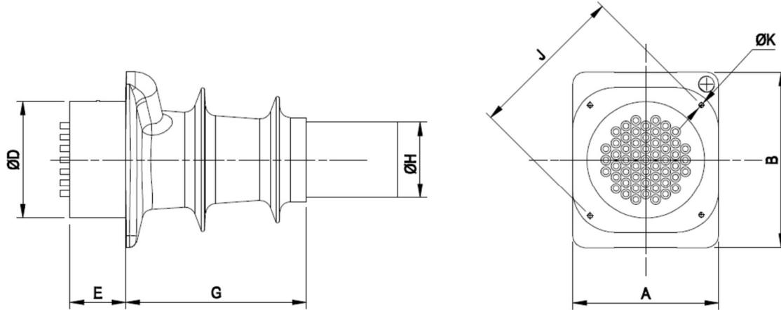
Figure 42 Anchorages type NC and NC-U @53/64 MPa dimensions
