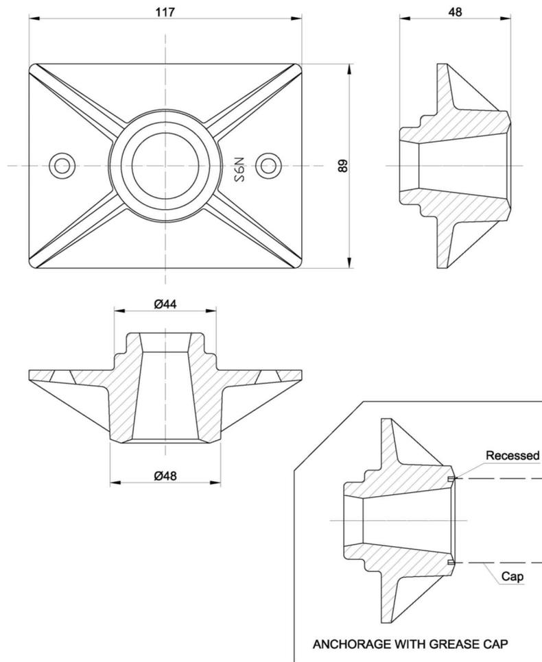
**Figure 65 Anchorage body type S 6-1 Standard**
