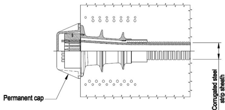
Figure 40 Categories of use arrangements anchorage type NC and NC-U
