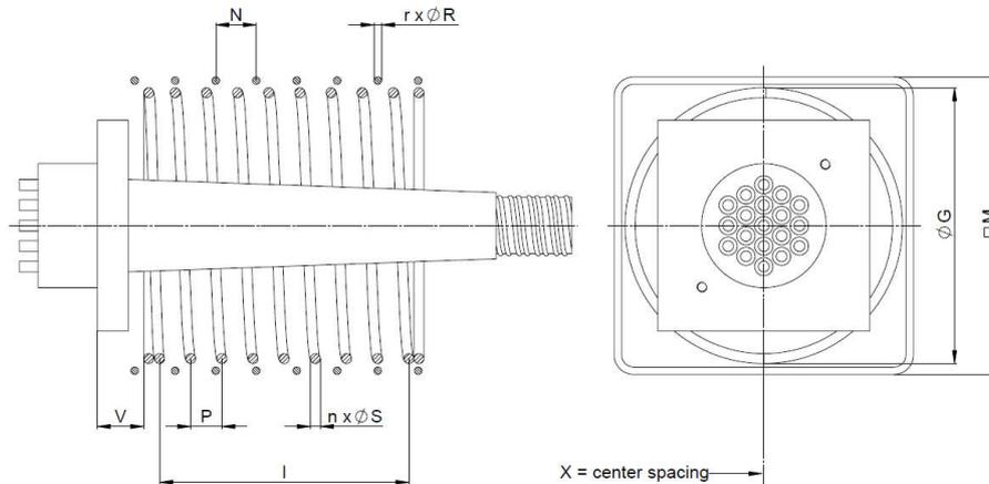
Figure 27 Local anchorage zone reinforcement type E @ 32/40 MPa
