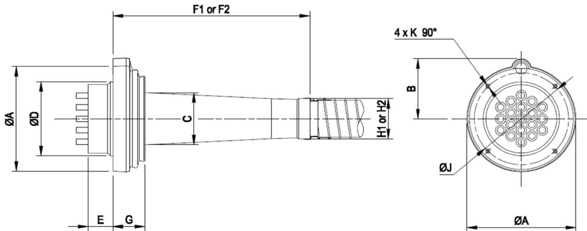
Figure 32 Anchorages type CS @28/35 MPa dimensions
