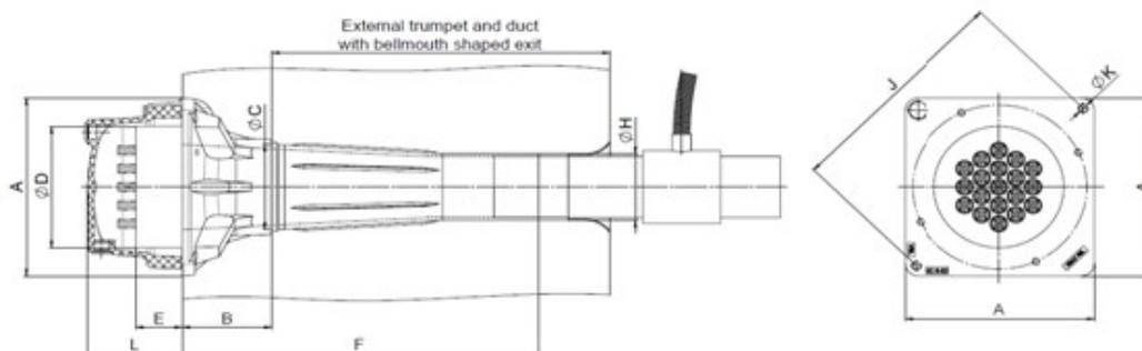
Figure 36 Anchorages type GC external tendons dimensions
