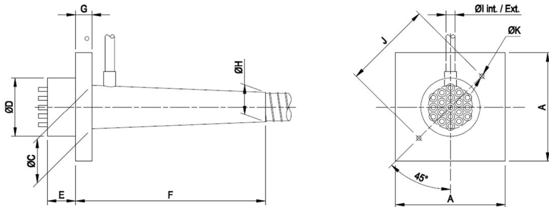
Figure 20 Anchorages type E @ 43/53 MPa dimensions
