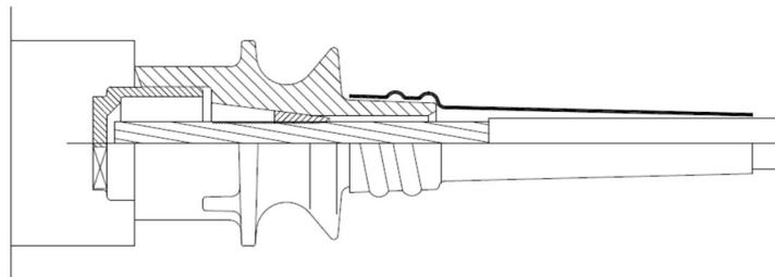
**Figure 55 Anchorage type S 6-1 - Unbonded system**
