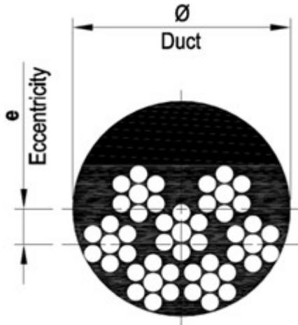
Figure 50 Ducting dimensions
