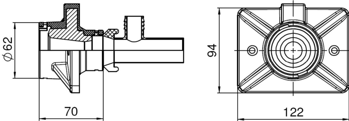
**Figure 61 Anchorages type S 6-1 PLUS - Dimensions**
