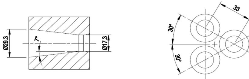
**Figure 8 Hole detail anchor head type CS**
