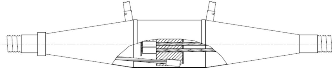
Figure 47 Category of use arrangement couplers type V
