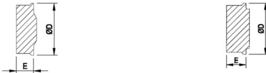
**Figure 10 Cross section anchor head type CS**
