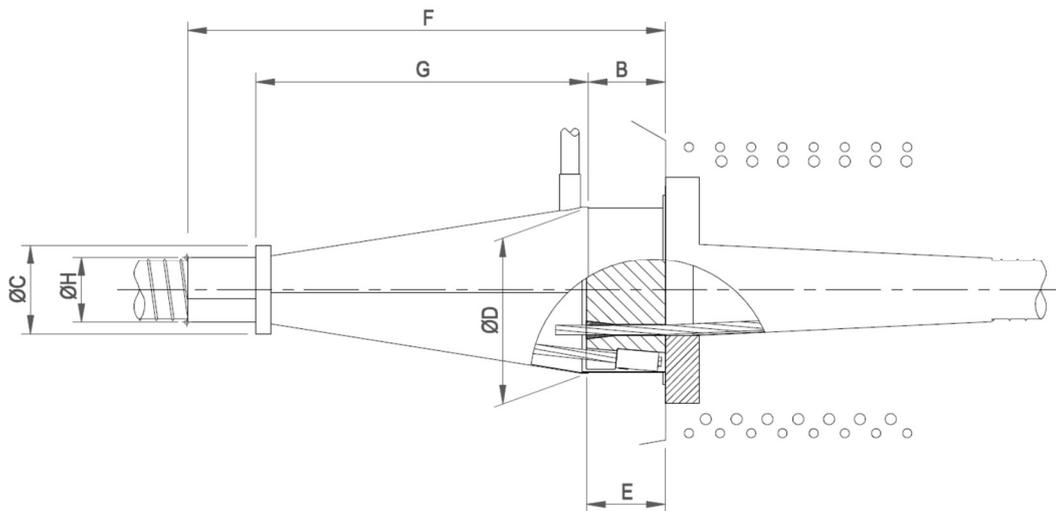
Figure 46 Couplers type K dimensions
