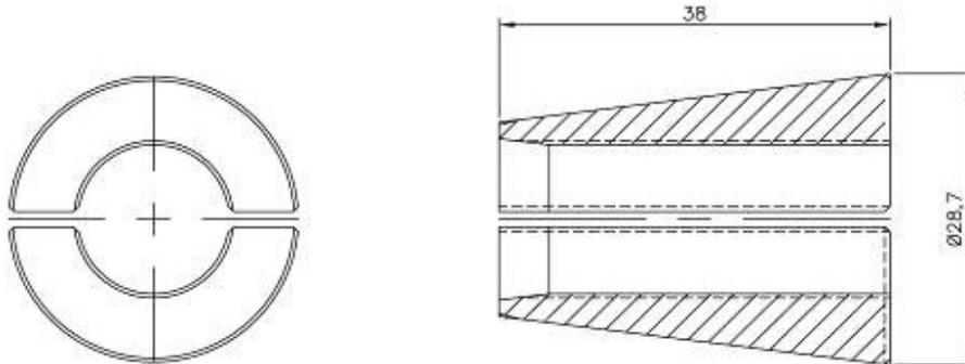
**Figure 53 Wedge W6M (for use with T15.2 strand)**
