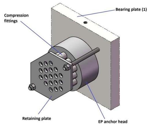
Figure 13 Categories of use arrangements anchorage type E
