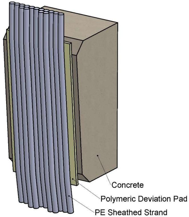
**Figure 16 Deviator E-WT – Flat deviator**
