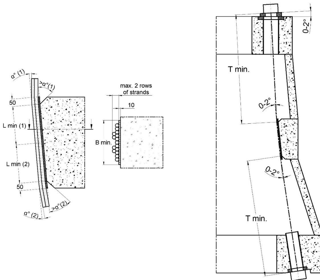
**Figure 23 Deviator E-WT – Flat deviator - Geometry and dimensions**
