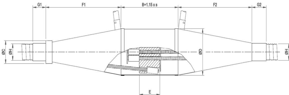
Figure 48 Couplers type V dimensions
