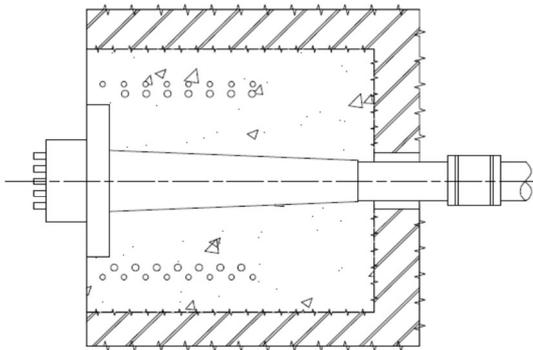
Anchorage placed against steel structure
