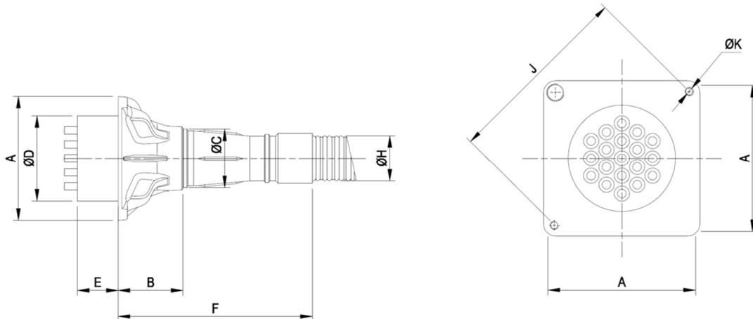
Figure 35 Anchorages type GC standard bonded post-tensioning dimensions
