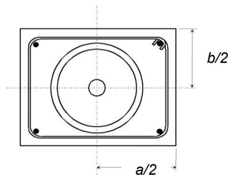
$a/2$  and  $b/2$  are the distances between the anchorage axis and the edge of the test specimen.
