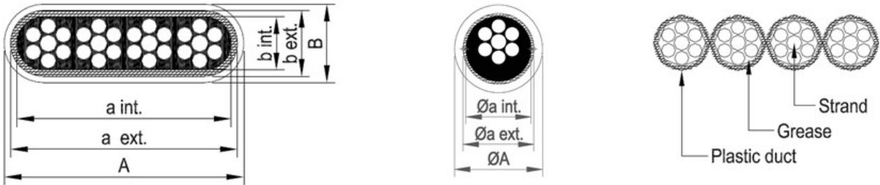
**Figure 85 VSL PT-PLUS® Duct bonded / bonded / unbonded**
