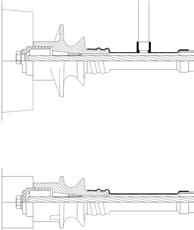
**Figure 56 Anchorage type S 6-1 - Bonded system**
