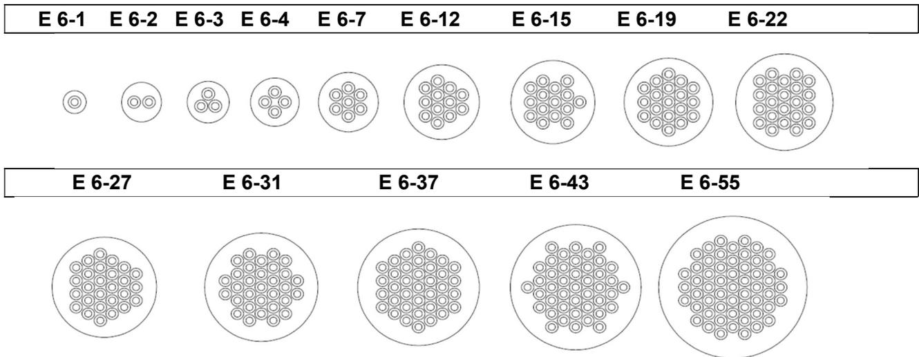
**Figure 6 Hole spacing anchor head type E**
