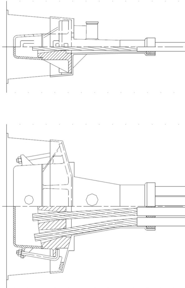
**Figure 70 Anchorage type S 6-4 - Unbonded system**
