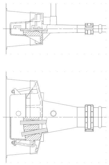
Figure 71 Anchorage type S 6-4 - Bonded system
