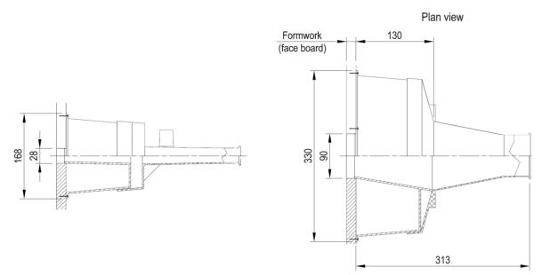
Figure 73 Anchorages type S 6-4 – Dimensions of placing devices
