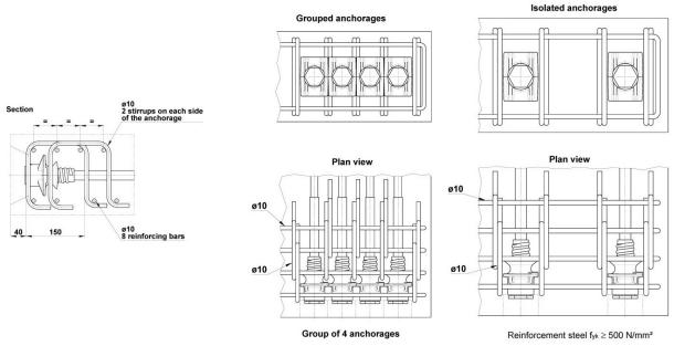
Figure 74 Example of additional reinforcement to combine with main one type S 6-1  $f_{c,min}(t)$ >16/20 N/mm<sup>2</sup>
