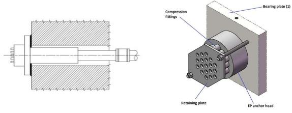
Figure 13 Categories of use arrangements anchorage type E
