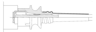
Figure 55 Anchorage type S 6-1 - Unbonded system
