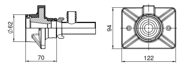
Figure 61 Anchorages type S 6-1 PLUS - Dimensions
