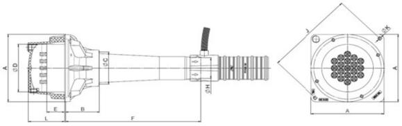
Figure 37 Anchorages type GC electrically isolated tendons dimensions
