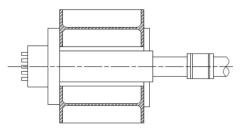
Anchorage with EP anchor head
