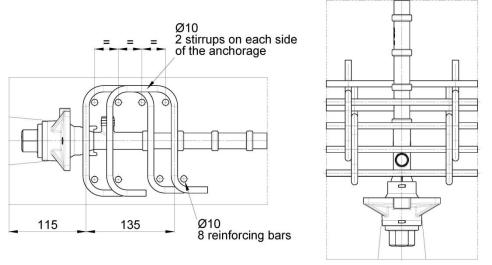
Reinforcement steel  $f_{yk} \ge 500 \text{ N/mm}^2$
