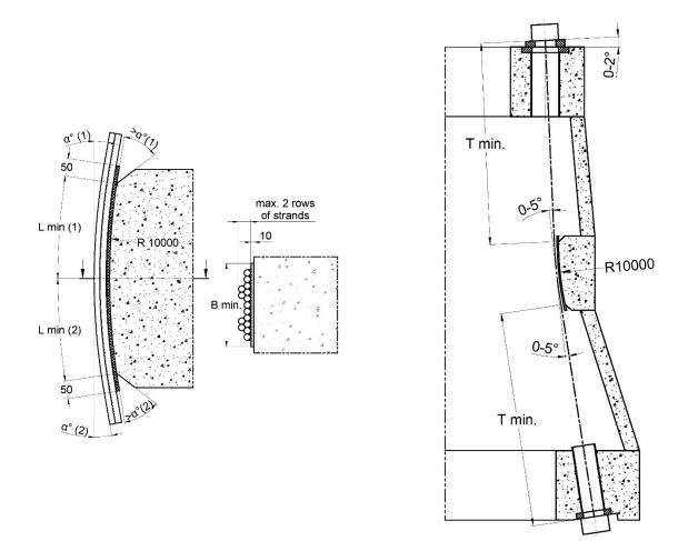
Figure 24 Deviator E-WT – Curved deviator - Geometry and dimensions
