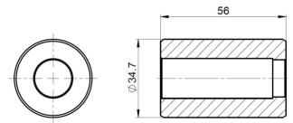
Figure 2 Compression fitting CFE6
