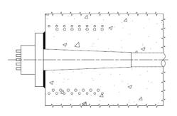
Anchorage placed against concrete structure
