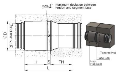
Figure 51 Segmental Couplers – PT-Plus Round Duct
