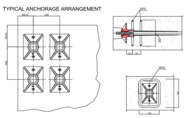
Figure 76 Example of additional reinforcement to combine with main one type S 6-1 PLUS and S 6-1 Standard f<sub>c,min</sub>(t)>20/25 N/mm2
