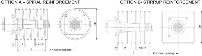
Figure 39 Local anchorage zone reinforcement type GC external and electrically isolated tendons
