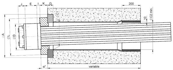
Figure 22 Anchorage type E-WT - Arrangement with shim plate - Dimensions
