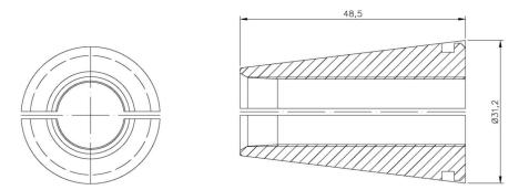
Figure 54 Wedge W6ML (for use with spring-loaded coupler)
