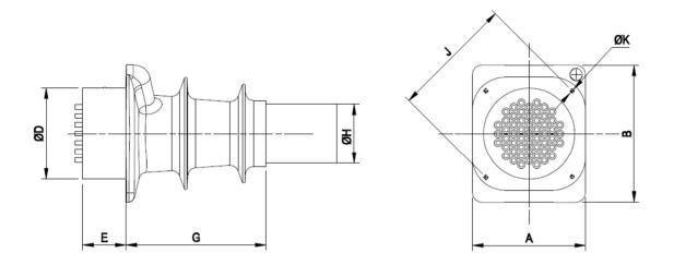
Figure 42 Anchorages type NC and NC-U @53/64 MPa dimensions
