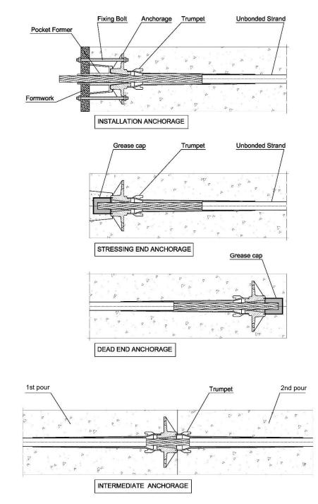
Figure 63 Anchorages type S 6-1 Standard - Unbonded system
