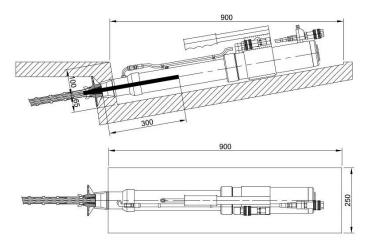
Figure 84 Clearance requirements with jack Alevin A7-24
