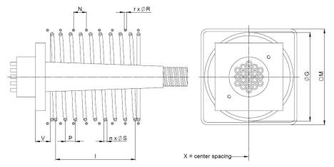
Figure 29 Local anchorage zone reinforcement type E @ 43/53 MPa
