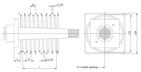
Figure 26 Local anchorage zone reinforcement type E @ 28/35 MPa
