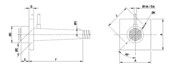
Figure 19 Anchorages type E @ 32/40 and 36/45 MPa dimensions
