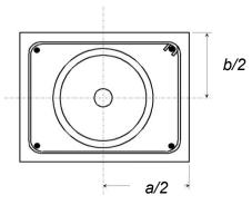
a/2 and b/2 are the distances between the anchorage axis and the edge of the test specimen.
