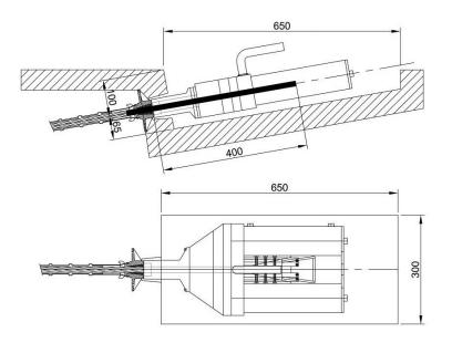
Figure 83 Clearance requirements with Twin jack 25T
