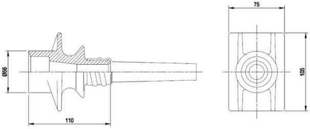
Figure 57 Anchorages type S 6-1 - Dimensions
