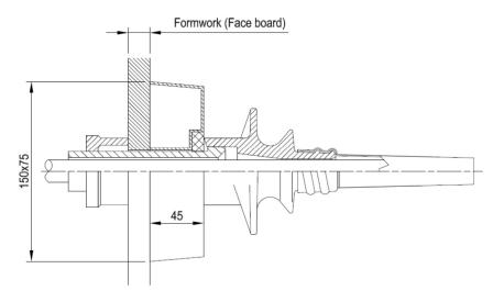
Figure 58 Anchorages type S 6-1 – Dimension of placing devices
