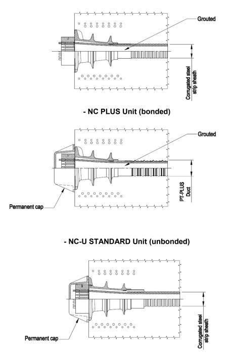
Figure 40 Categories of use arrangements anchorage type NC and NC-U
