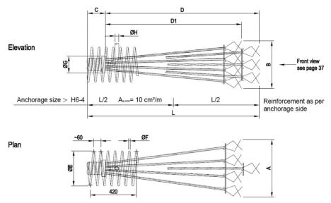
Figure 44 Anchorage and local anchorage reinforcement type H @ 28/35 MPa
