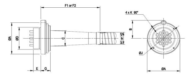
Figure 32 Anchorages type CS @28/35 MPa dimensions
