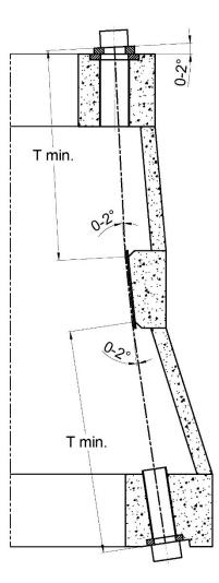
Figure 23 Deviator E-WT – Flat deviator - Geometry and dimensions
