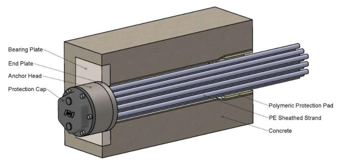
Figure 14 Anchorages type E-WT (External unbonded tendons)-Arrangement without shim plate
