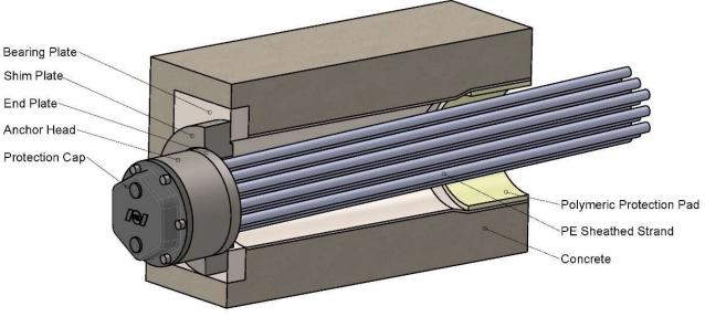
Figure 15 Anchorages type E-WT (External unbonded tendons)-Arrangement with shim plate
