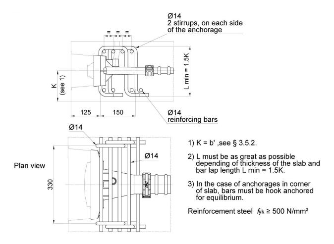
Figure 77 Example of additional reinforcement to combine with main one type S 6-4 f<sub>c,min</sub>(t)>16/20 N/mm<sup>2</sup>
