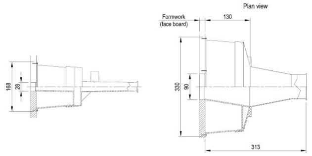
Figure 72 Anchorages type S 6-4 - Body and sleeve dimensions
