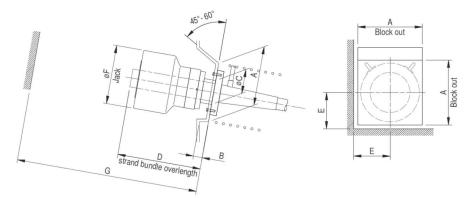
Figure 49 Block-out dimensions – Clearance requirements
