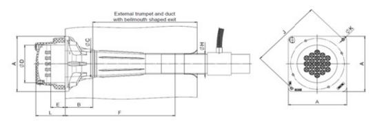
Figure 36 Anchorages type GC external tendons dimensions
