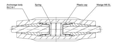
Figure 69 SK 6-1 SL Spring loaded coupler assembly drawing
