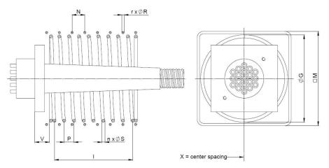
Figure 25 Local anchorage zone reinforcement type E @ 23/28 MPa
