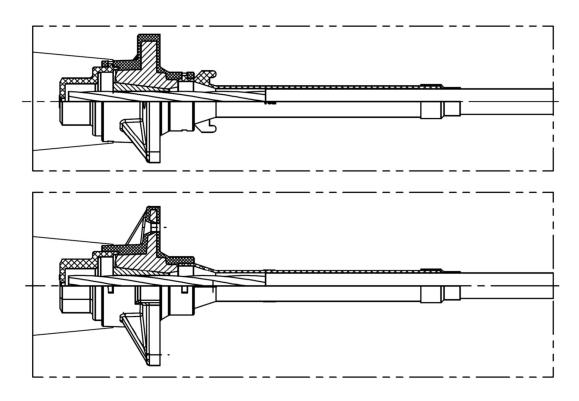
Figure 59 Anchorage type S 6-1 PLUS - Unbonded system
