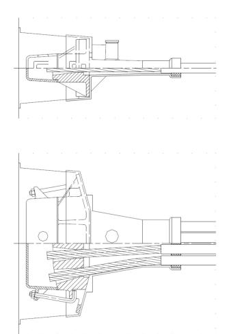
Figure 70 Anchorage type S 6-4 - Unbonded system
