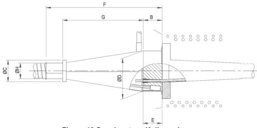
Figure 46 Couplers type K dimensions
