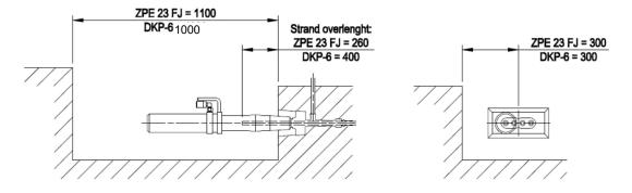
Figure 82 Clearance requirements with jacks DKP-6 and ZPE 23FJ
