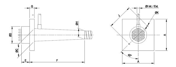
Figure 18 Anchorages type E @ 23/28 and 28/35 MPa dimensions
