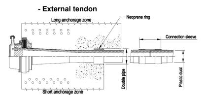
Figure 31 Arrangements anchorage type CS external tendon
