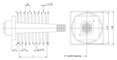
Figure 27 Local anchorage zone reinforcement type E @ 32/40 MPa
