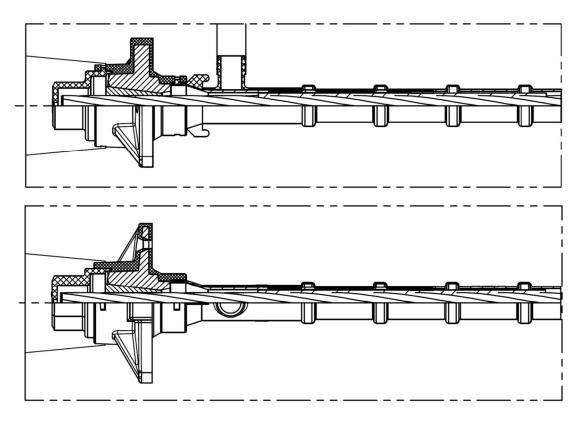
Figure 60 Anchorage type S 6-1 PLUS - Bonded system
