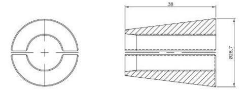
Figure 53 Wedge W6M (for use with T15.2 strand)
